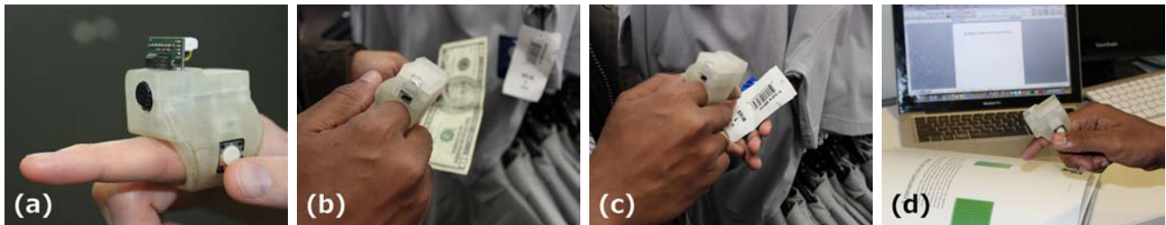
Figure 1. EyeRing: A finger-worn input device. (a) EyeRing prototype. (b) CurrencyDetector application. (c) TagDetector application. (d) Interaction with printed media.
