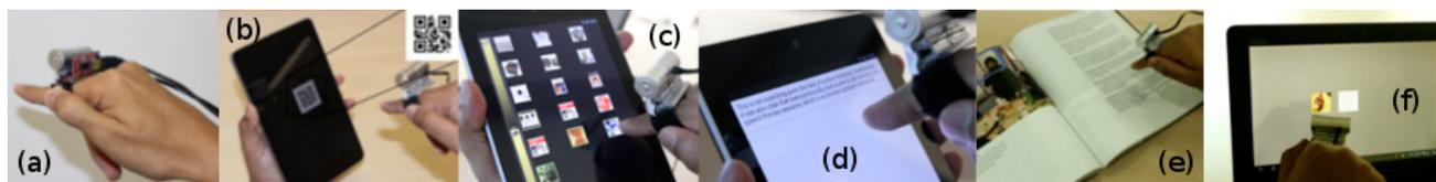
Figure 1. SmartFinger; (a) current prototype (b) connecting to a digital device (c) copying digital media (d) extracting a part of digital document (e) extracting contents from a physical document (f) pasting selectively
