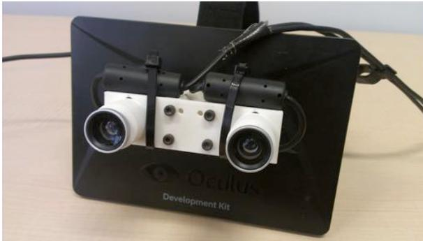
**Figure 2. Stereoscopic video-see-through HMD.**
